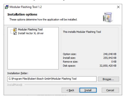
ModularFlashingTool installation needs ~120 MB free disk space on the local hard disk. >> Press button "Install" to continue or Cancel to abort the installation.
